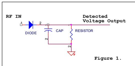
The detected output voltage which is an average of the RF sample is fed either directly to a meter movement or conditioned before being fed to an analog or digital display. The diode detection method shown above will work well for CW type signals and fairly narrow band signals with low crest factors.
